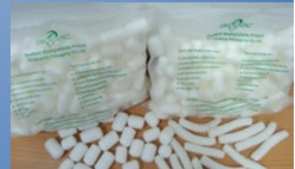
Starch-based foam which 100% biodegraded by microorganisms in soil
